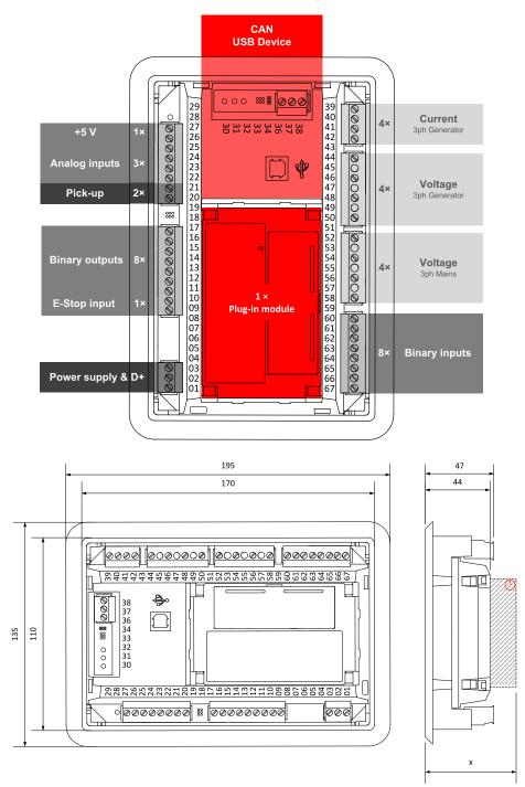
**Note:** The final depth of the controller depends on the selected plug-in module – it can vary between 41 mm and 56 mm. Mind also the size of connectors and cables (e.g. in case of RS232 connector, add about 60 mm more for standard RS232 connector and cable).
